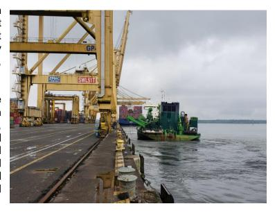
A total of 206,000 m³ of dredged sediments were transferred through 68 cycles or trips to the sea, at a distance of 37 kilometers from the project area; final dumping site duly approved and authorized by the competent environmental and maritime authorities, for which the "LANGE WAPPER" suction dredger was used with a capacity of 13,700 m³ in the hopper.
